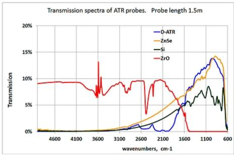
Specification of IR-Fiber HT-ATR-Probes for High Temperatures FlexiSpec®
