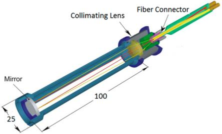
Specification of Gas Transmission Fiber Optic Probes FlexiSpec®
