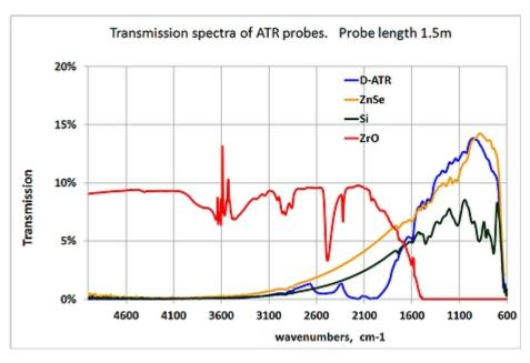
Specification of Fiber Optic Immersion ATR- Probes FlexiSpec®
