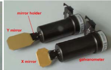
Mounted scan mirror with galvo
